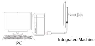
Connect the USB port of the integrated machine to the USB port of the computer. Set the working parameters of the integrated machine using DEMO software.
