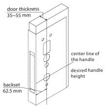
Note 1: Align the template along the vertical center line of the mortise (G) at the desired handle height, and tape it to door.
