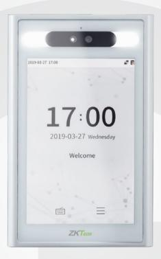
**Elite Access** is a new high-level facial recognition terminal with extremely powerful facial recognition capability supported with ZKTeco's customized powerful CPU and ultra-large capacity of facial templates, a maximum of 50,000 facial templates for 1:N recognition.
