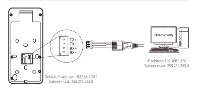
Click [COMM.] > [Ethernet] > [IP Address], input the IP address and click [OK].
