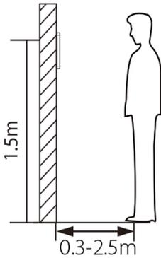
The distance between the device and a user whose height is within 1.55m-1.85m is recommended to be 0.3-2.5m. Users may slightly move forwards and backwards to improve the quality of facial images captured.
