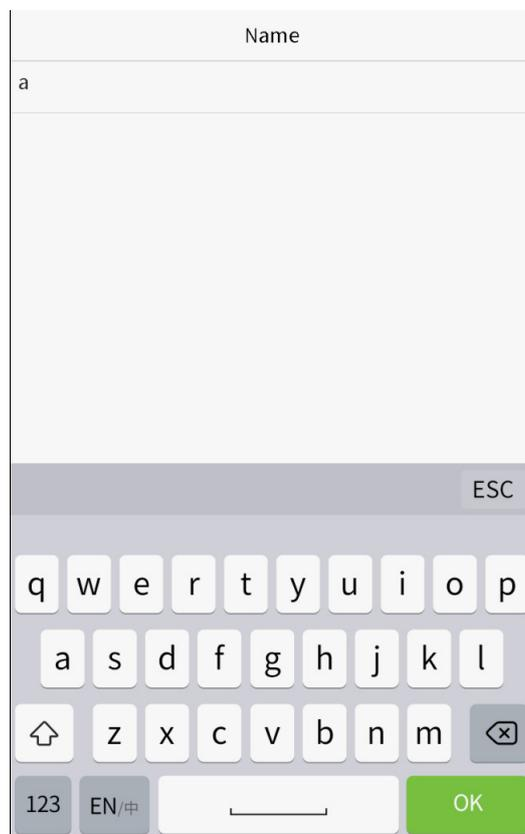
**Note:** The device supports the input of Chinese, English, numbers and symbols. Click [**En**] to switch to English keyboard. Press [**123**] to switch to the numeric and symbolic keyboard, and click [**ABC**] to return to the alphabetic keyboard. Click the input box, virtual keyboard appears. Click [**ESC**] to exit the input.
