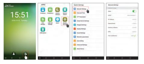
Go to Main Menu > System Settings > Network Settings, set the IP Address. The device will communicate with PC via the Ethernet parameters. Using Cloud Service Settings sets Server Address and Server port according to the server.
