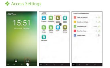
Go to Main Menu > Access Settings > Access control parameters to enter Access control parameters setting interface.
