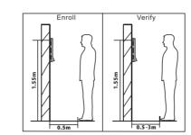
The registration and verification position of the device should not be changed to avoid affecting the verification accuracy. If it is necessary to move the device, then move it horizontally and keep the vertical height same.
