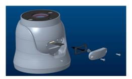
Step 4, close the cover and tighten the screws.
