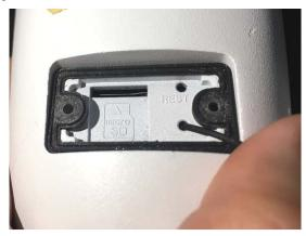
Step 3, install the Micro-SD card in the correct direction and insert it into the slot.
