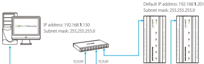
**Note:** In LAN, IP addresses of the server (PC) and the device must be in the same network segment when connecting to the software.
