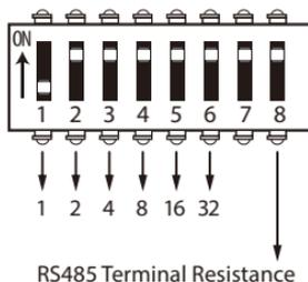
1. Number 1-6 are reserved to set the device number for RS485 communication. The code is binary, and the numbering starts from left to right. When the switch is set to ON position, it indicates 1 (on); when the switch is set downwards, it indicates 0 (OFF).
