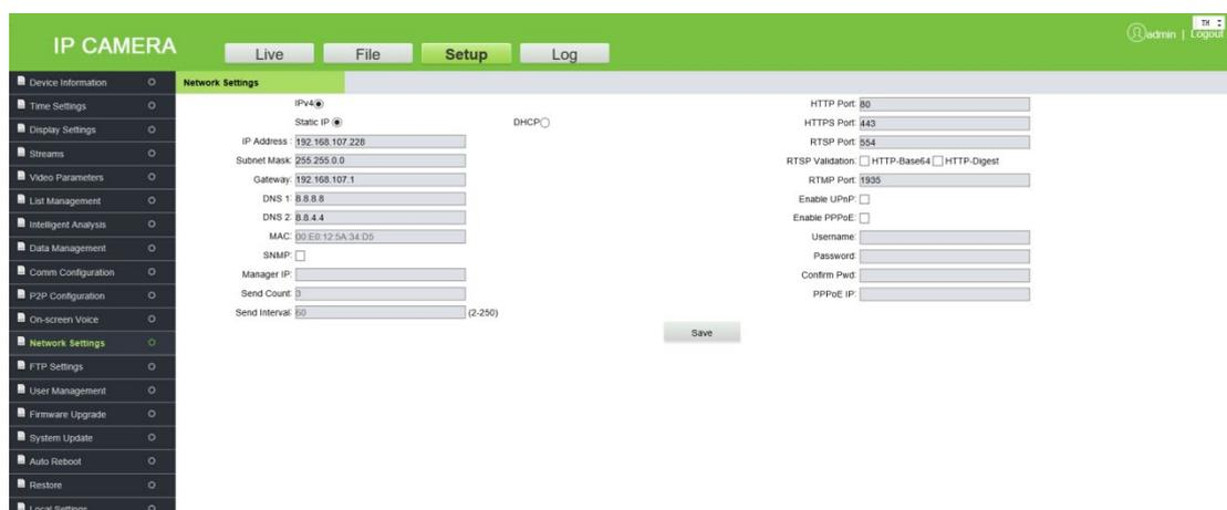
**LAN:** Set the related parameters of the Local Area Network, including IP Address, Subnet Mask, Gateway, DNS, and MAC according to the actual situation, click [**Save**].
