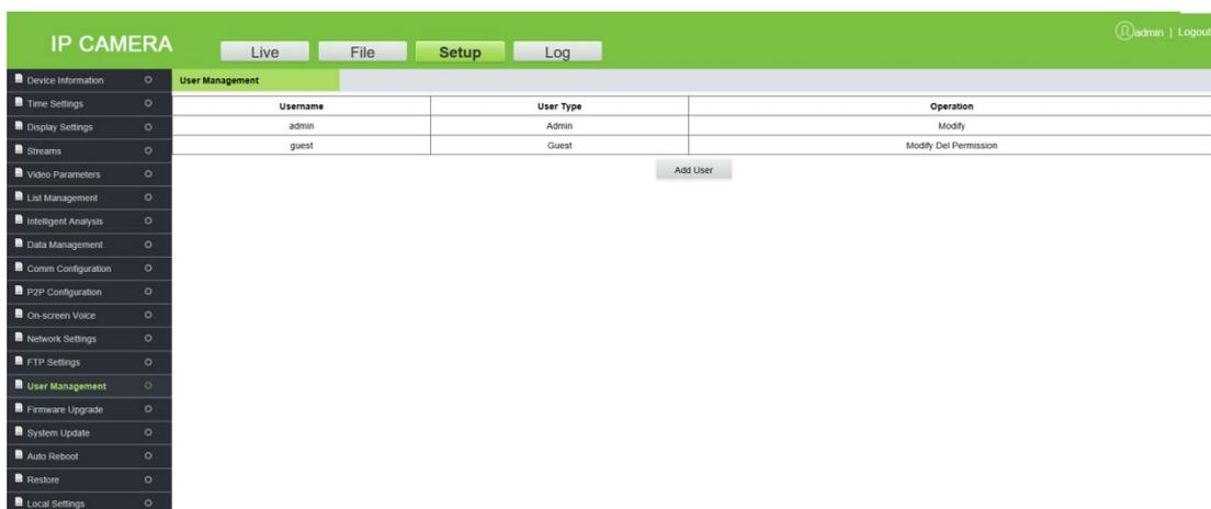
**Modify:** Modification preferences vary with different stages of users, where passwords can be modified only for administrators, and user type can be modified for normal users. The Username, Password, and user type can be modified for a new user by the administrator. New users can be set as a normal user or operator. Different permissions can be assigned in "Permissions".
