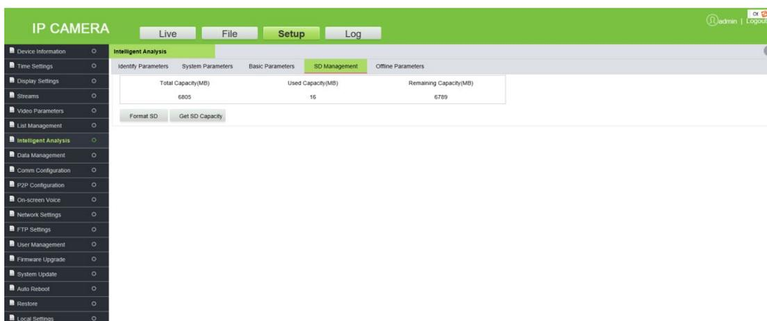
When the camera uses an SD card, this tab shows the total space, used space and remaining space of the SD card. You can format and re-use the SD card.
