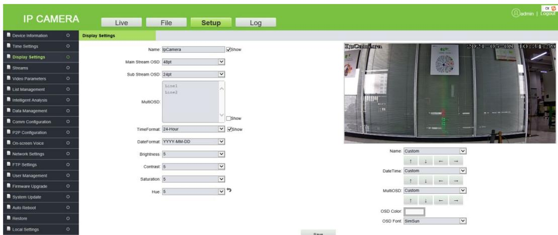
**Name:** The user can change the name of the specific channel to a maximum of 31 bytes in length. Upon selecting the 'Show' check box, it will appear on the preview screen.
