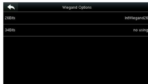
Set the Wiegand format matching the card module of the device. After a unified Wiegand format is used, correct card numbers can be read. The Wiegand format can be set to **IntWiegand26**, **IntWiegand26a**, **IntWiegand34**, or **IntWiegand34a** so that card numbers read by the device are in the preset format.
